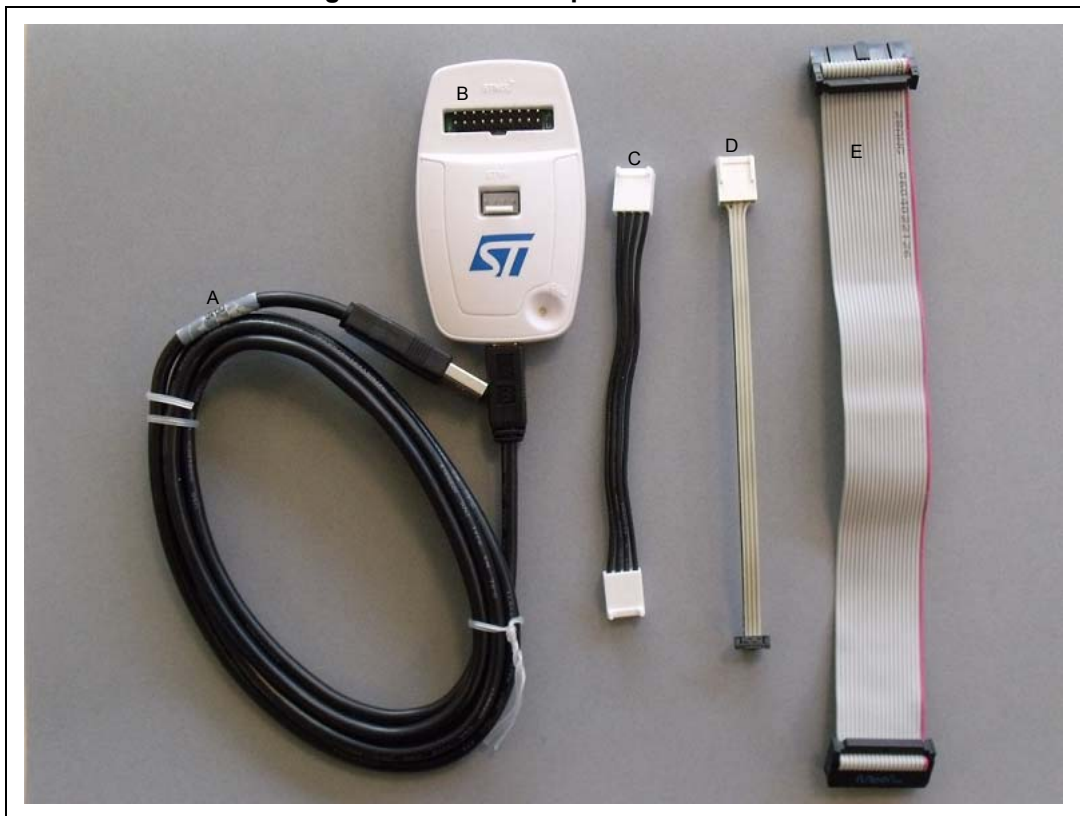
Figure 2. ST-LINK/V2 product contents
