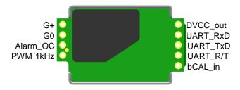
Figure 2. Diffusion Pin assignment
