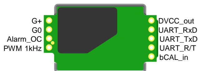
Figure 2. Diffusion Pin assignment
